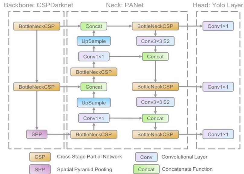
Fig. 9. The network architecture of Yolov5.
