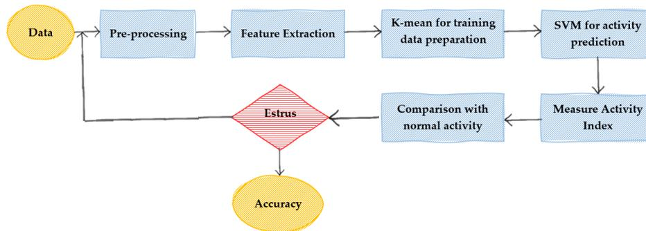
Fig. 4. System flow diagram of estrus detection.
