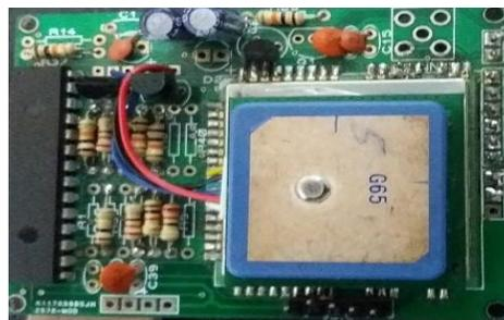
**Fig. 1.** Data-logger circuitry with mounted GPS.
