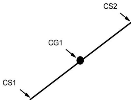
Fig. 6: Link coordinate system
