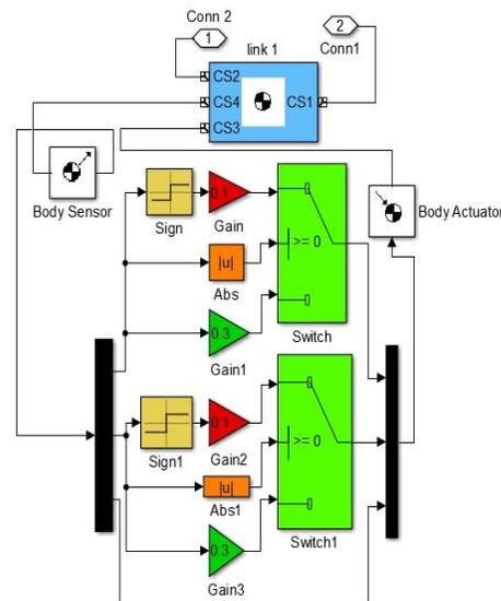
Fig. 7: Coulomb's friction module of an individual link
