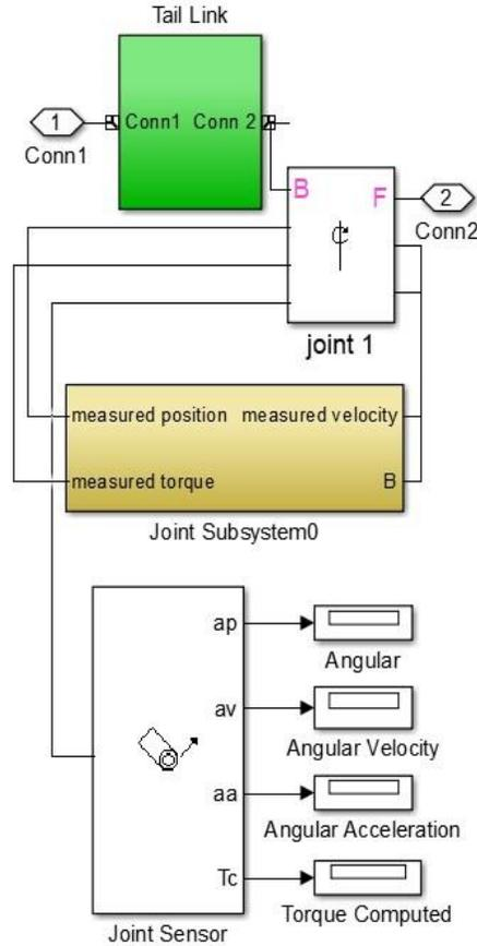
Fig. 4: Link joint subsystem of 10-link snake robot
