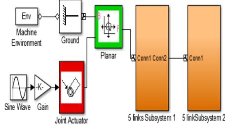
Fig. 3: Snake robot in a Simmechanics environment
