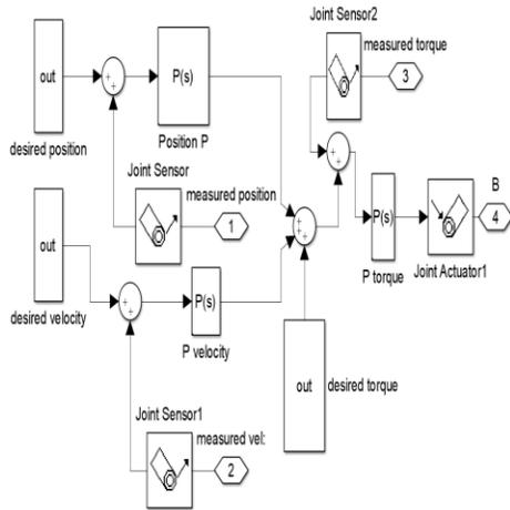
Fig. 5: Joint control subsystem
