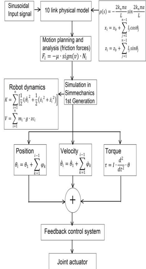
Fig. 1: System Block Diagram of a 10-link Snake Robot
