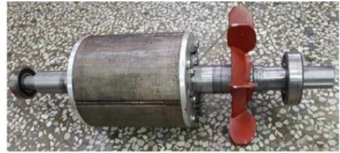
(c) Assembled rotor with shaft, fan and bearing before machining
