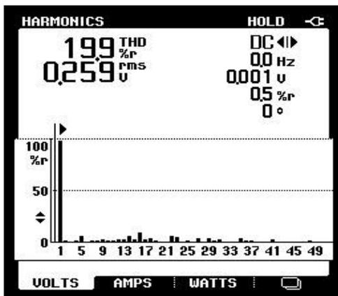
Fig 10(e): THD of filtered output Voltage
