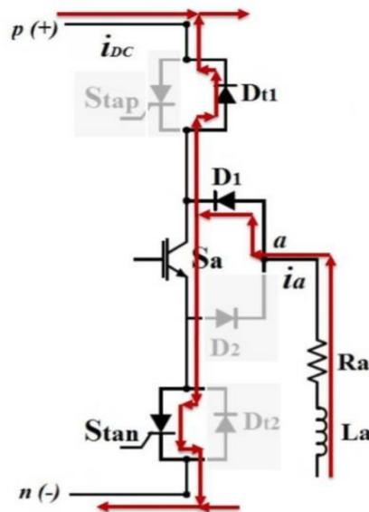
Fig 3(b): Current Control Scheme for Single Phase
