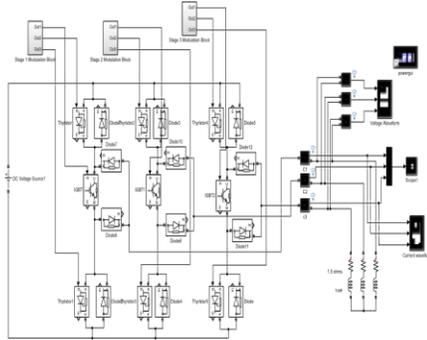
Fig 7: MATLAB/Simulink Model of VSI
