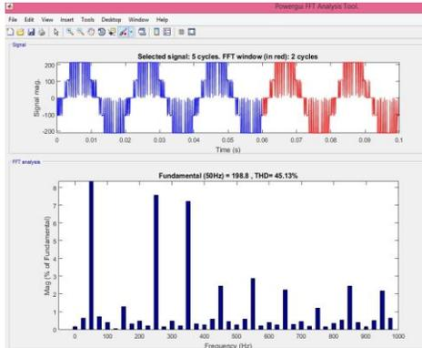
Fig 8(a): THD of Voltage Waveform without Filter
