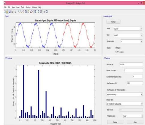
Fig 8(c): Current THD with RL load without filter
