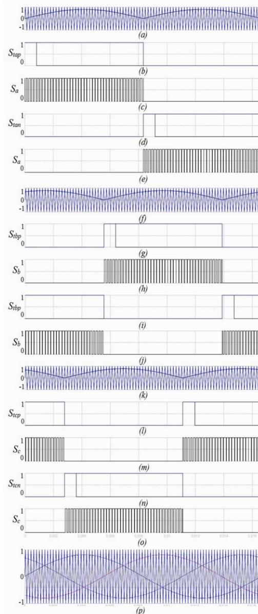
Fig 6: Switching Control Scheme for stage 1, 2 and 3
