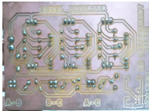
**Fig 10(b):** Circuit Design on PCB Board
