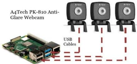
Fig. 6 Raspberry Pi-4 connected with 03nos. of Web-Cams
