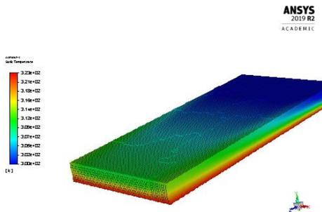
Fig 12: Temperature contours of solar glass surface after water cooling
