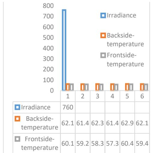
Fig 6: Front and backside temperatures of modules at higher irradiance
