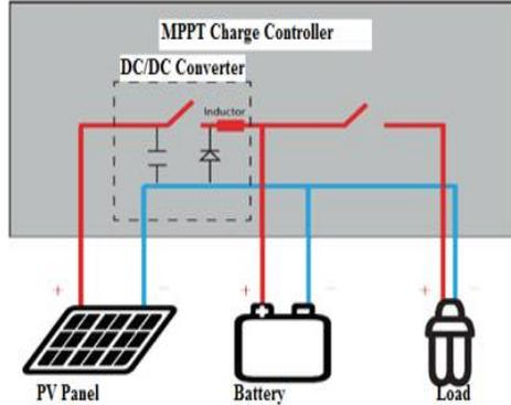
**Fig 3:** MPPT charge controller
