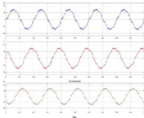
Fig 8(b): Output Current Waveform without Filter
