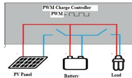
Fig 1: PWM charge controller
