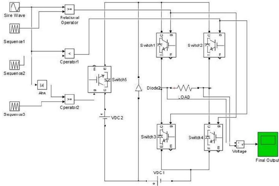
**Fig. 11.** Single phase of Five level multilevel inverter
