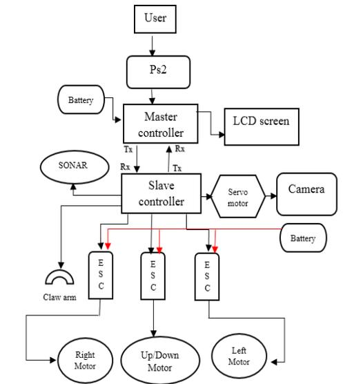
**Fig. 5.** Flow chart of UUV
