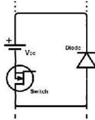
**Fig. 2.** Unit cell of the proposed Asymmetric cascaded MLI
