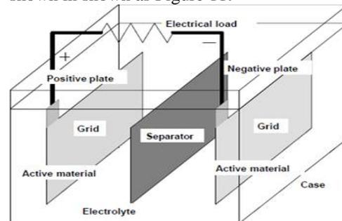
**Fig 11:** Lead Acid Battery
