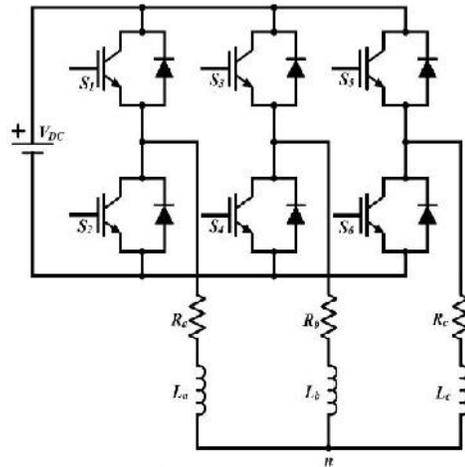
Fig 1: Schematic model of proposed topology
