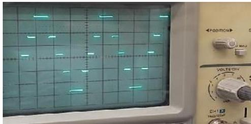
**Fig. 21.** Single phase output of MLI prototype
