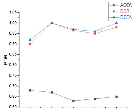
Fig 2: Packet delivery Ratio of AODV, DSDV, DSR
