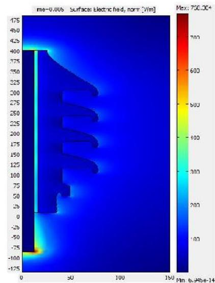
Fig. 4. Simulated electric field distribution in transformer bushing.
