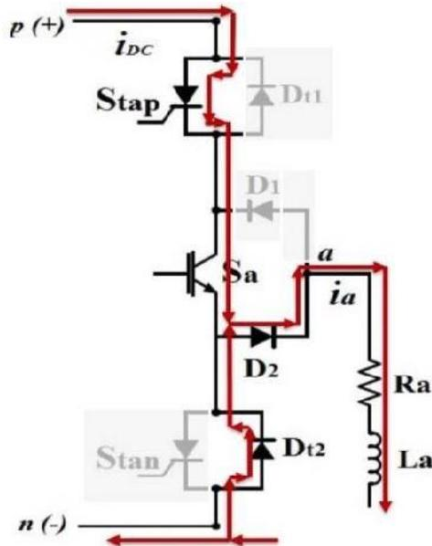
Fig 3(a): Current Control Scheme for Single Phase
