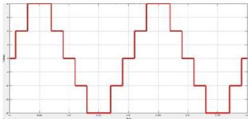
**Fig. 13.** Simulation results five level single Phase Multilevel Inverter
