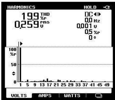
Fig 10(e): THD of filtered output Voltage
