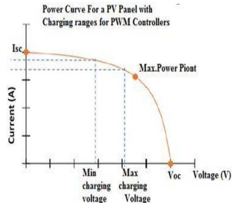
Fig 2: Power curve for PWM controller
