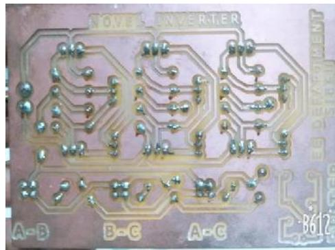
**Fig 10(b):** Circuit Design on PCB Board
