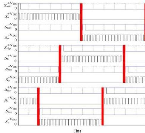
Fig 5. Conduction sequences of devices
