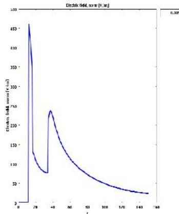
**Fig. 5.** Cross-sectional view of electric field in the bushing model
