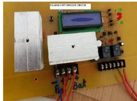
**Fig 16:** Solar Charge Controller
