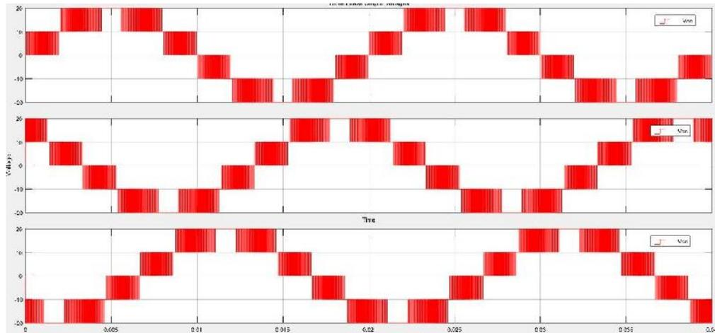
Fig. 16. Three Phase MLI SPWM Modulated Output
