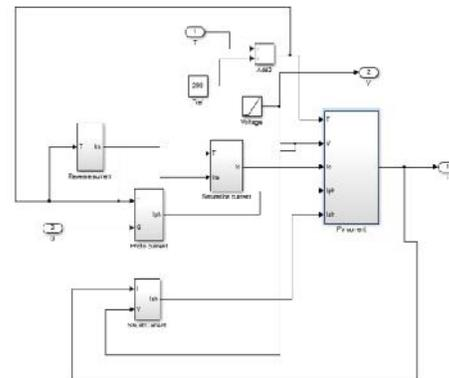
**Fig 6:** Grouped Subsystem of PV module
