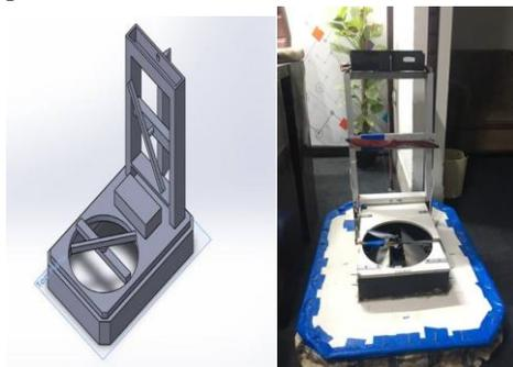
**Fig. 1:** Hovercraft CAD structure prototype and final
