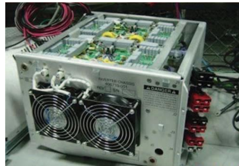
Fig 3: High voltage chassis consist of two transformers having secondary of 140kV.
