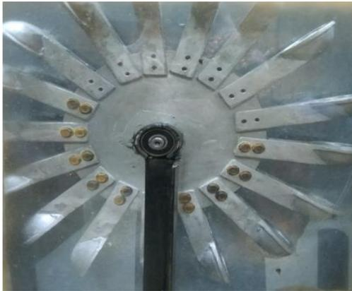
Fig 7: Pelton Turbine in the casing
