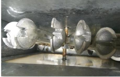
Fig 8. Buckets of Pelton Turbine
