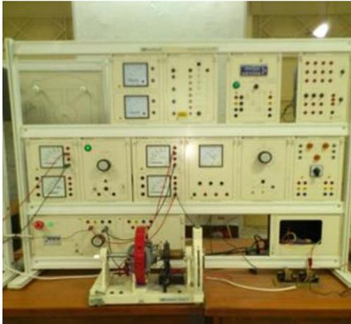
Fig 7: Experimental setup of DC Series Motor with Armature Controller
