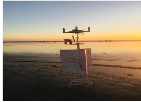
Fig. 6. IoT based Tidal Energy Transducer at the Arabian Sea
