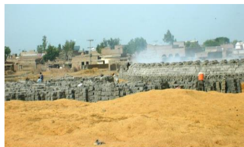
Fig. 4. Rice husk used in brick manufacturing industries [40]
