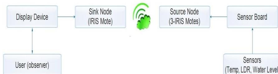
Fig. 2. Block diagram of the system
