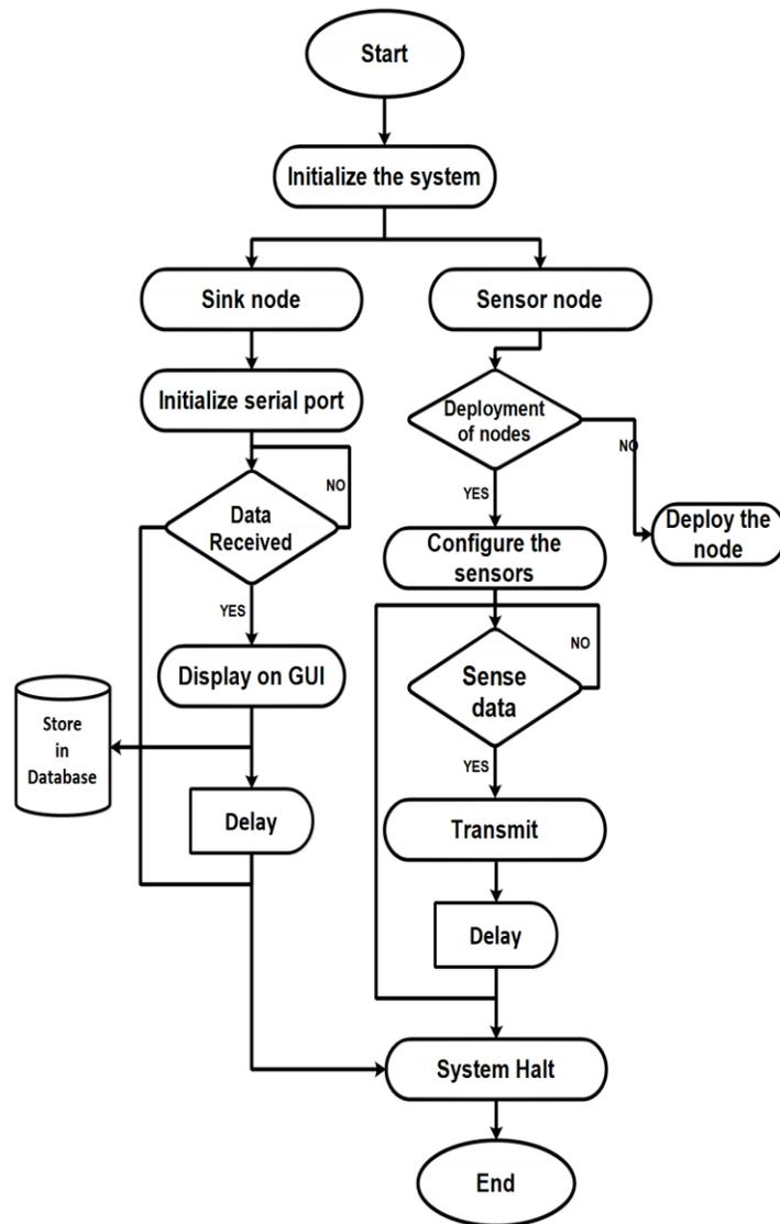
Fig. 5. Flowchart for sink and sensor nodes
