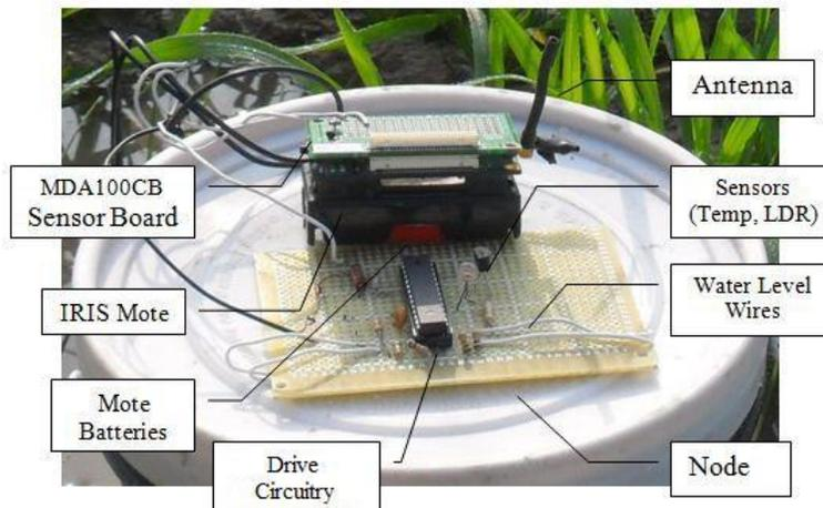
**Fig. 3.** Complete picture of a sensor node
