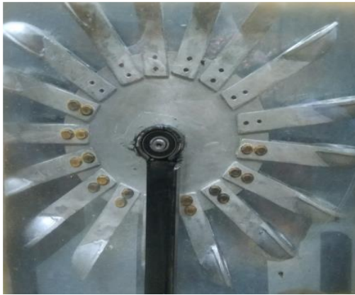
Fig 7: Pelton Turbine in the casing
