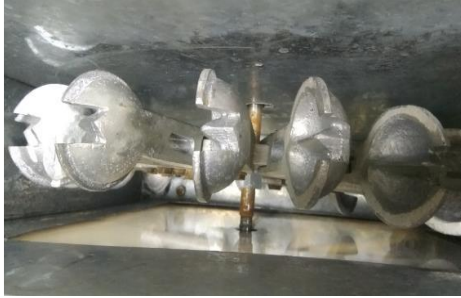
Fig 8. Buckets of Pelton Turbine
