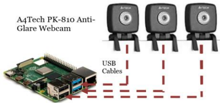
Fig. 6 Raspberry Pi-4 connected with 03nos. of Web-Cams
