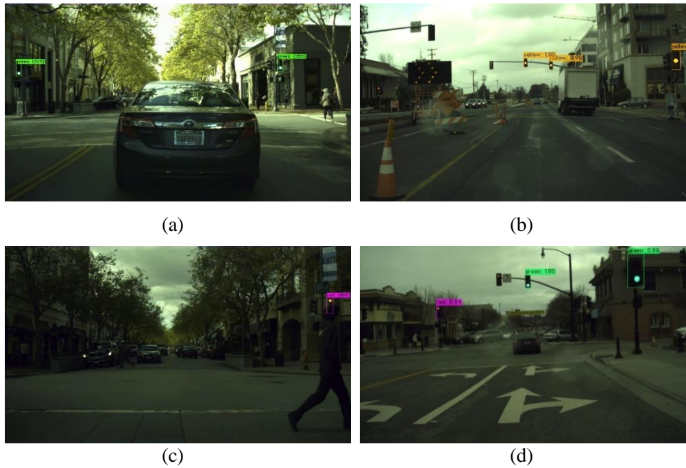
Fig. 7. Output Images YOLO V3 in different lighting conditions. (a) Green light detection (b) Yellow light detection (c) Red Light detection (d) Misc. lights detection
