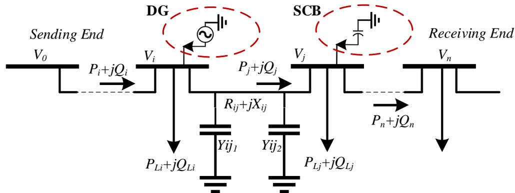
**Fig. 1.** One line of typical radial feeder
