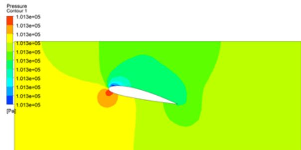
**Fig. 13.** Pressure plot across airfoil at 12.6 degrees angle of attack inside test section
