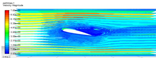
**Fig. 10.** Path-lines of air across airfoil in the test section
