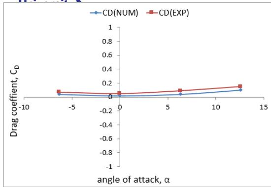
**Fig. 8.** Numerical and Experimental plots of NACA-2414 Drag coefficient
