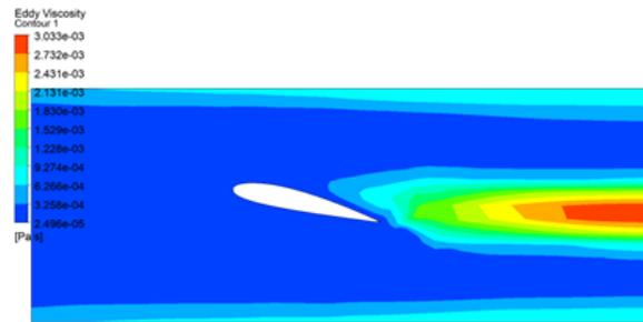
**Fig. 12.** Eddy Viscosity Contour plots across wind tunnel test section
