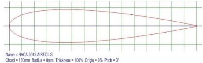
Fig. 3. Airfoil NACA-0012 plot profile [14]
