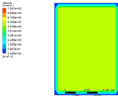
**Fig. 9.** Contour velocity plot across wind tunnel outlet test section
