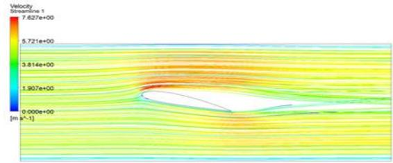
**Fig. 11.** Streamline plot with balls representing the path of streamlines at test section
