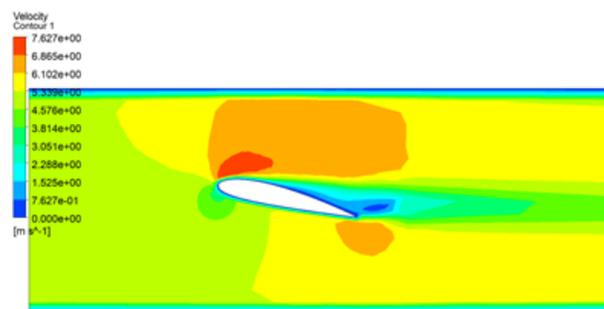
**Fig. 14.** Velocity plot across airfoil at 12.6 degrees angle of attack inside test section
