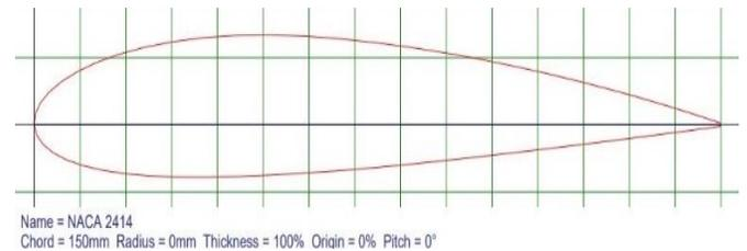
Fig. 4. Airfoil NACA-2414 plot profile [14]
