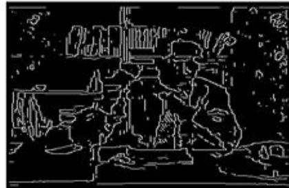
Figure 2: Objects detection Using Canny algorithm
